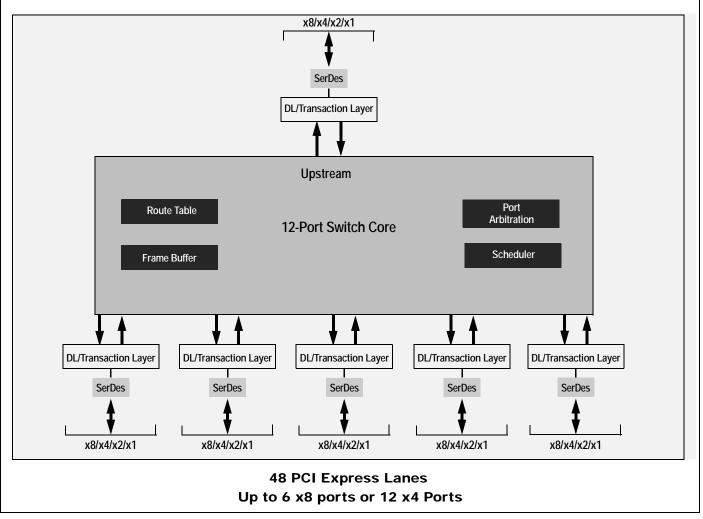
Figure 1 PES48T12 Block Diagram
