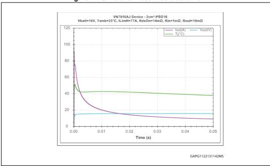
Figure 44. Simulation result-cold condition
