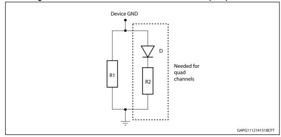
Figure 24. Recommended GND network for ISO 7637-2 (2011) level IV
