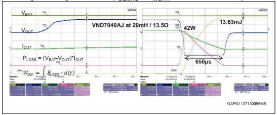
Measured T<sub>DEMAG</sub>: 6500 µs (633 µs calculated)
