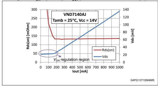
Figure 50. R<sub>ON</sub> dependency on I<sub>OUT</sub> (measured on a VND7140AJ sample)
