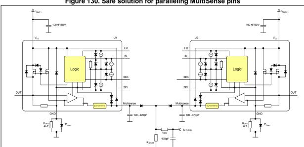
Figure 130. Safe solution for paralleling MultiSense pins
