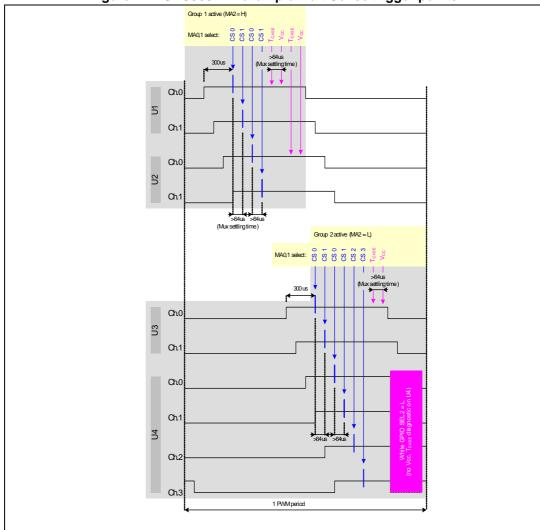
Figure 117. SPC560Bxx example MultiSense trigger points
