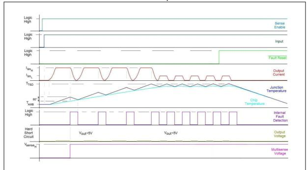
Figure 28. Latch functionality - behavior in hard short circuit condition (autorestart mode and latch-off)
