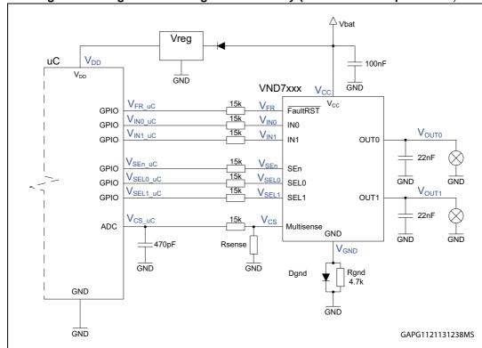
Figure 3. Voltage levels during reverse battery (diode + resistor protection)
