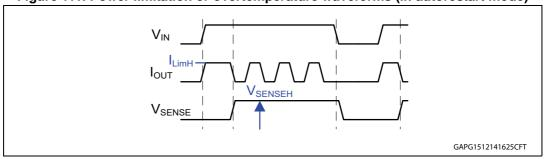
Figure 112. Power limitation or overtemperature waveforms (in lacth mode)
