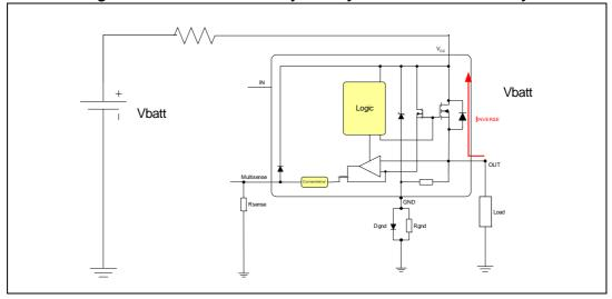
We define I<sub>INVERSE</sub> the current that flows into the device from the output.
