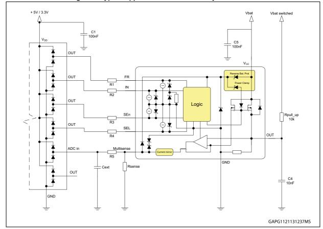
Figure 2. Typical application schematics - hybrid devices
