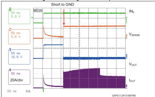
Figure 94. Failure flag indication-example 4
