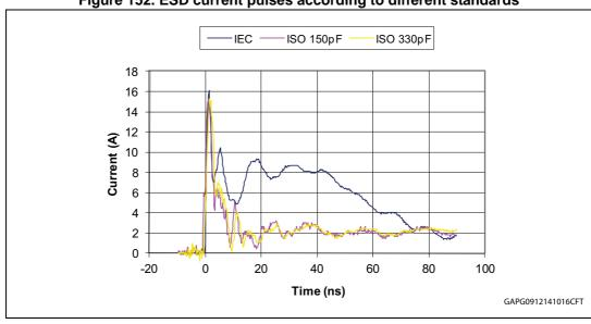
Figure 152. ESD current pulses according to different standards
