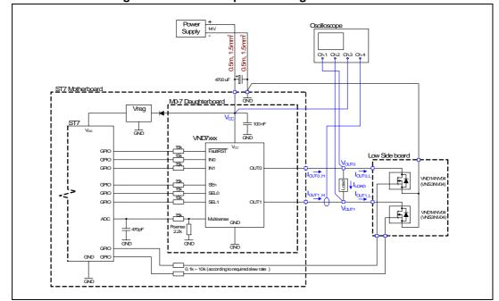
Figure 162. Test set up for H-Bridge cross current
