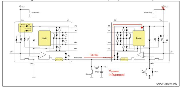
Figure 132. Direct connection of MultiSense pins (not recommended)
