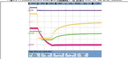
Figure 7. Measurement example ( $t_{DEMAG} > t_{D-STBY}$ ) with 4.7 k $\Omega$  GND resistor
