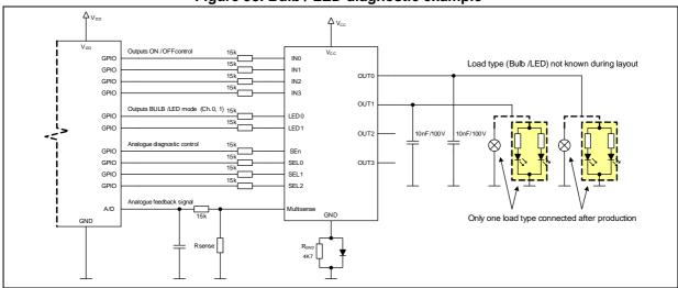
Figure 98. Bulb / LED diagnostic example
