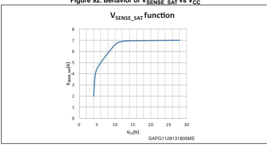
Figure 92. Behavior of V<sub>SENSE SAT</sub> vs V<sub>CC</sub>
