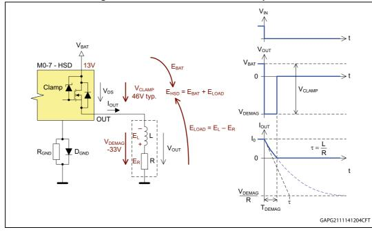
Figure 73. Inductive load-HSD turn-off phase
