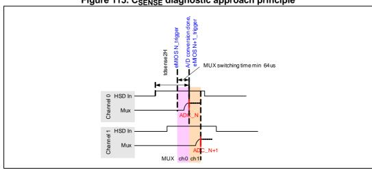
Figure 115. C<sub>SENSE</sub> diagnostic approach principle
