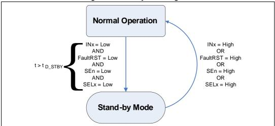
Figure 30. Standby state diagram
