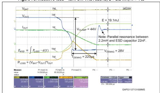
Figure 76. Inductive load – turn-off: VND7020AJ, L = 2.2 mH, R = 4  $\Omega$
