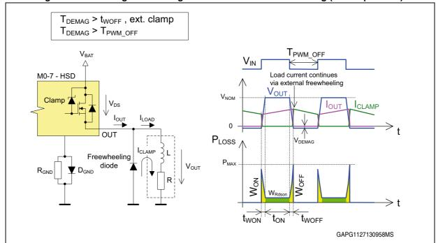
Figure 63. Switching losses - high inductance + ext. freewheeling (PWM operation)
