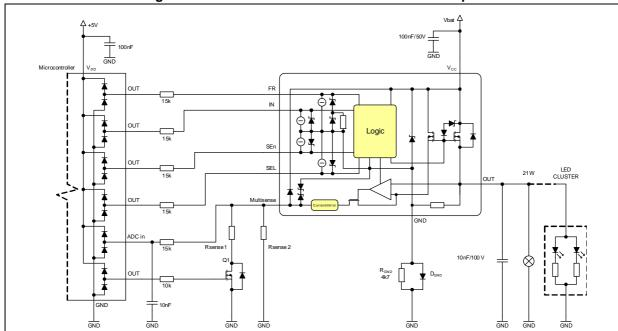
Figure 100. Switched current sense resistor-example
