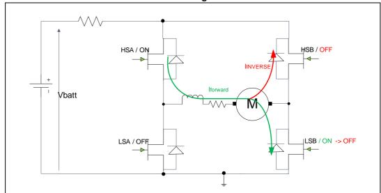
Figure 148. Inverse Current injected by an inductive load in the high-side driver of an H-Bridge
