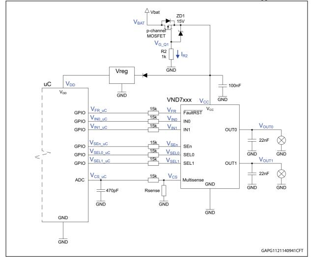
Figure 11. Generic schematic and test setup with P-channel MOSFET in V<sub>CC</sub> line
