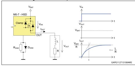
Figure 71. HSD turn-on phase with inductive load
