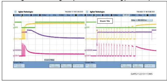
Figure 31. FR handling example - bulb inrush blanking (VNQ7140AJ)
