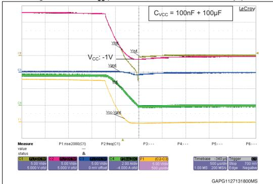
Figure 87. Loss of  $V_{CC}$  (VND7020AJ, 1 mH/ 3.5  $\Omega,$  100 nF + 100  $\mu\text{F})$
