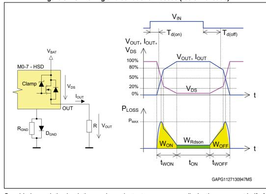
Figure 51. Switching and conduction losses (resistive loads)
