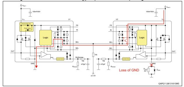
Figure 127. Direct connection of SE<sub>n</sub> pins (not recommended) during loss of GND
