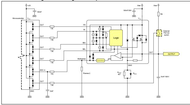
Figure 105. Analogue HSD - open load detection in off-state
