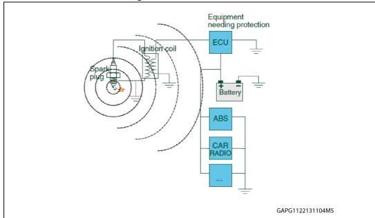
Figure 17. Radiated hazards
