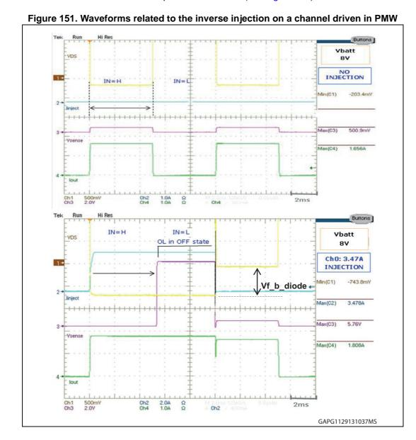
2. Device state: ChUT in PWM. Test execution: Increasing Inverse Current is injected in a channel (the ChUT) up to the I<sub>INVERSE</sub> while the ChUT is driven ON
