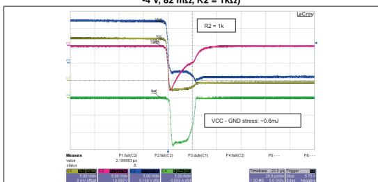
Figure 13. Reverse battery test according to LV 124:2009-10: VN7016AJ (13.5 V at -4 V, 82 m $\Omega$ , R2 = 1k $\Omega$ )
