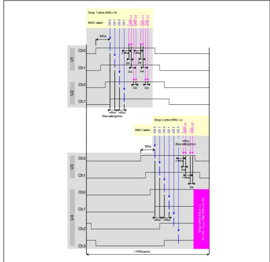
Figure 122. GND shift measurement position example
