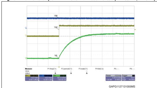
Figure 72. Turn-on example: VND7140AJ with inductive load (L = 260 mH, R = 81  $\Omega$ )
