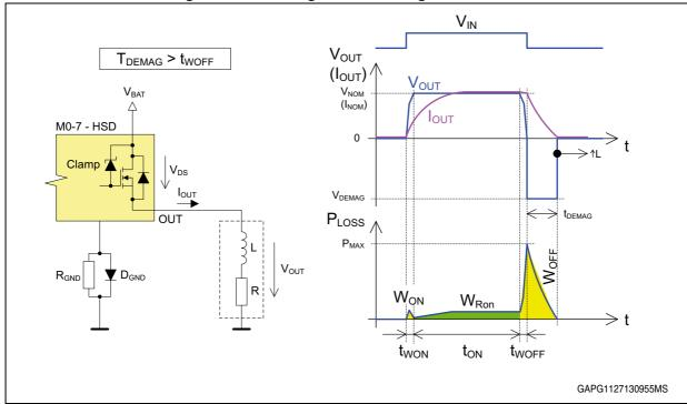
Figure 60. Switching losses with high inductance
