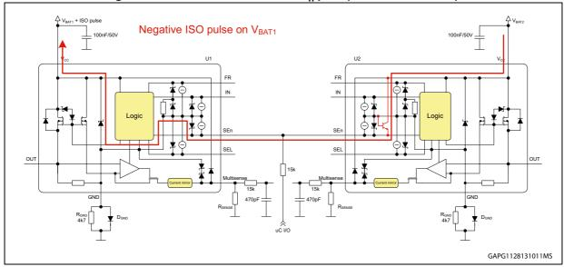
Figure 123. Direct connection of SE<sub>n</sub> pins (not recommended)
