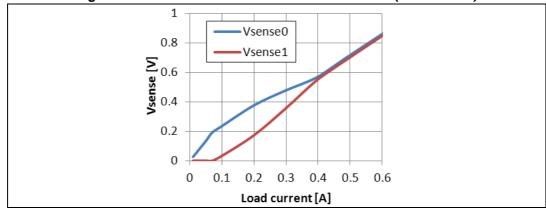
Figure 139. Current sense behavior at low current (VND7140AJ)
