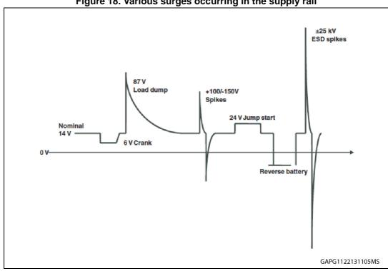
Figure 18. Various surges occurring in the supply rail
