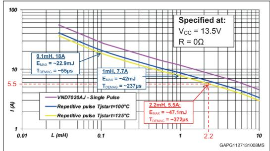
Figure 75. Maximum turn-off current versus inductance - VND7020AJ datasheet
