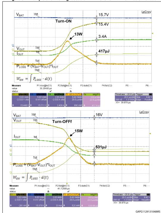
Figure 52. Example of switching losses on VND7040AJ with  $4.5\Omega$  resistive load
