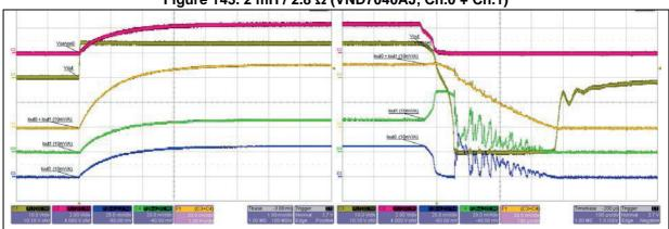
Figure 143. 2 mH / 2.8 Ω (VND7040AJ, Ch.0 + Ch.1)
