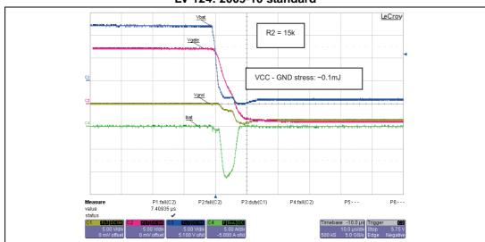
Figure 10. Reverse battery test VN7016AJ (13.5 V  $\rightarrow$  -4 V, 82 m $\Omega$ , R2 = 15 k $\Omega$ ) as per LV 124: 2009-10 standard
