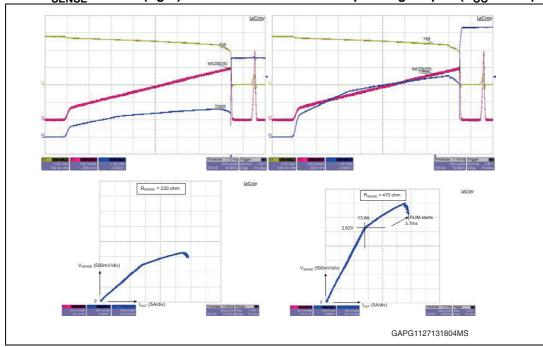
Figure 91. Plotted  $V_{SENSE}$  with increasing  $I_{OUT}$  versus time with  $R_{SENSE}$  = 220  $\Omega$  (left) and  $R_{SENSE} = 470 \Omega$  (right) for VND7040AJ and corresponding XY plot ( $V_{CC} = 14 \text{ V}$ )
