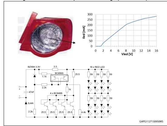
Figure 55. LED cluster example 2-tail & brake light (VW Passat B6)
