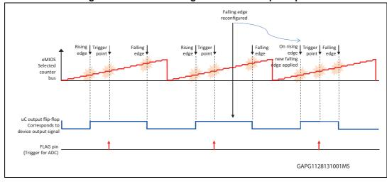
Figure 113. eMIOS PWM generation mode principle
