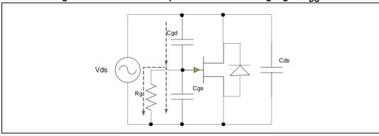
Figure 161. PowerMOS capacitance effect during high dV<sub>DS</sub>/dt
