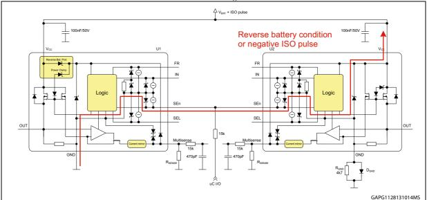
Figure 126. Direct connection of SE<sub>n</sub> pins (not recommended)
