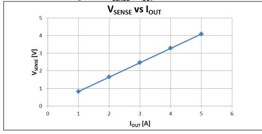
Figure 102. V<sub>SENSE</sub> vs I<sub>OUT</sub> measurement
