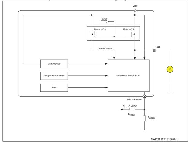
Figure 89. Structure of MultiSense signal generation
