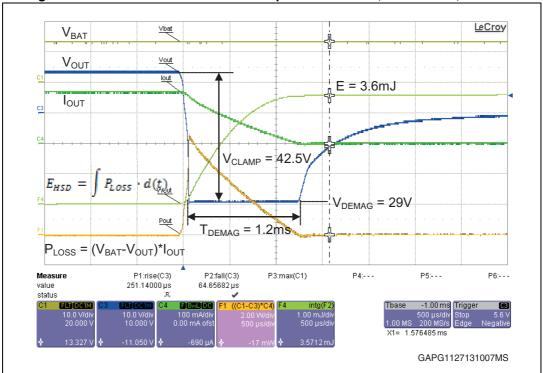
The demagnetization energy dissipated in the HSD was measured by an oscilloscope with mathematical functions. The first function F1 shows the actual power dissipation on the HSD ( $V_{BAT}$  -  $V_{OUT}$ ) \*  $I_{OUT}$ , the second function F4 shows the HSD energy (integral of F1).
