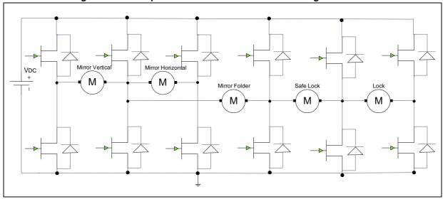
Figure 157. Example of automobile multi-motor driving connection
