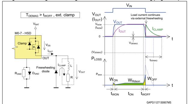
Figure 62. Switching losses with high inductance and external freewheeling (single event)
