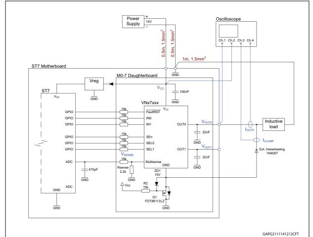
Figure 78. Test setup-verification of new external clamp proposal
