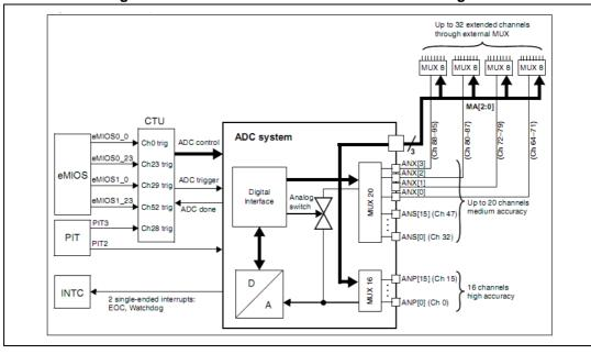
Figure 114. SPC extended ADC channels block diagram
