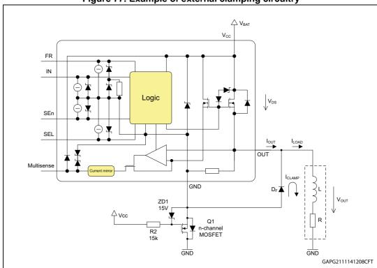
Figure 77. Example of external clamping circuitry
