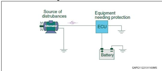
Figure 16. Conducted hazards
