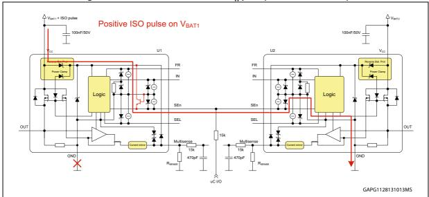
Figure 125. Direct connection of SE<sub>n</sub> pins (not recommended)
