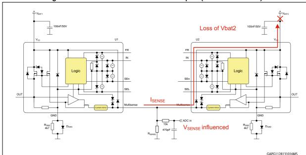
Figure 129. Direct connection of MultiSense pins (not recommended)
