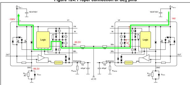
Figure 124. Proper connection of SE<sub>n</sub> pins
