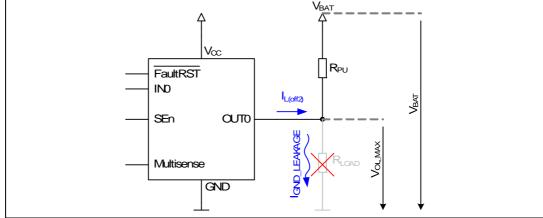
Resistor  $R_{PU}$  connected to  $V_{BAT}$  supply results to:
