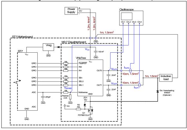
Figure 141. Test setup-paralleling of outputs (inductive loads)
