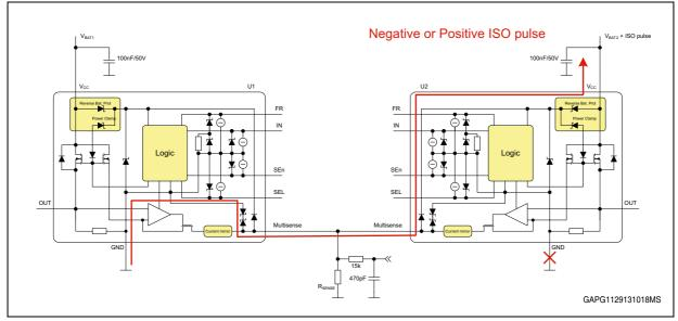
Figure 131. Direct connection of MultiSense pins (not recommended)
