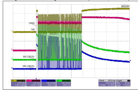
Figure 140. Behavior during overload condition (VND7040AJ, Ch.0 + Ch.1)
