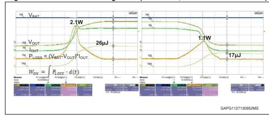
Figure 57. Slew rate and switching losses (VND7140AJ, VW Passat B6-tail & brake)
