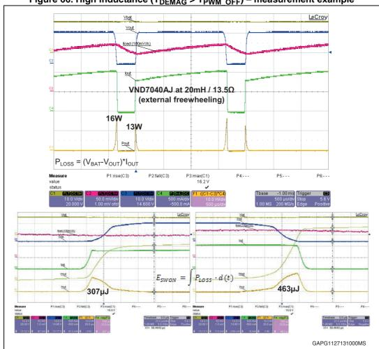
Measured losses (20 mH at 13.5  $\Omega):$   $W_{ON}$  ~ 307  $\mu J$  (I $_{OUT}$  ~ 1 A)
