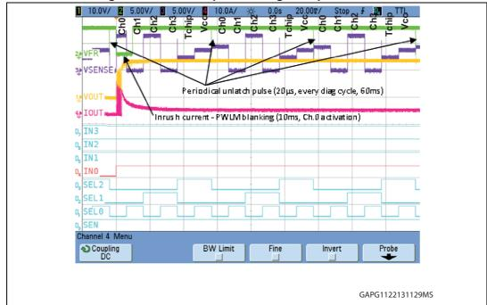
Figure 34. FaultRST pin handling example - overview
