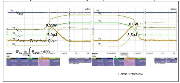
Figure 56. Slew rate and switching losses (VND7140AJ, LED test board)
