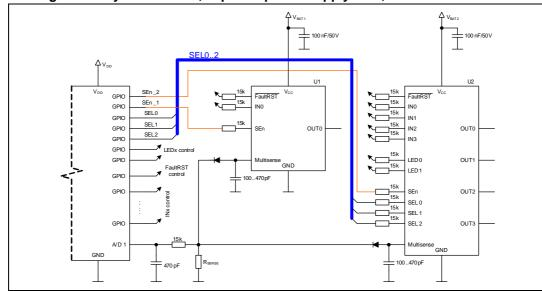
Figure 41. Hybrid devices, separate power supply rails, common MultiSense
