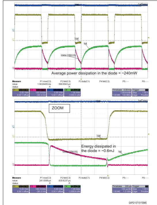
Figure 80. PWM 80 % at 400 Hz, 2 mH / 5.5 Ω (VND7040AJ)
