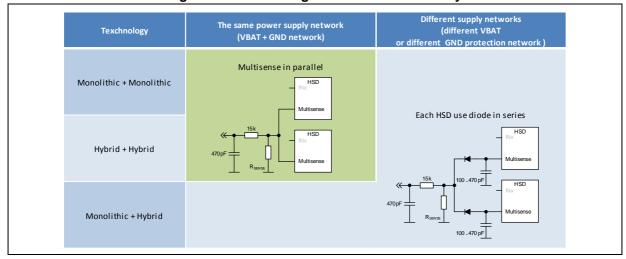
Figure 133. Paralleling of MultiSense summary
