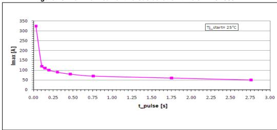
Figure 15. Maximum current versus duration time of VN5R003H-E
