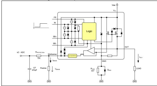
Figure 118. Low pass filter connection
