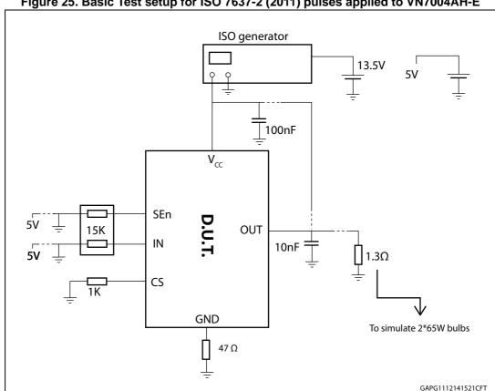
Figure 25. Basic Test setup for ISO 7637-2 (2011) pulses applied to VN7004AH-E
