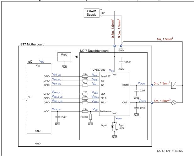
Figure 5. GND resistor requirements (inductive load)-test setup
