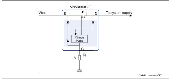
Figure 14. Reverse polarity protection – reverse FET protection
