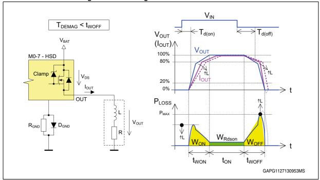
Figure 58. Switching losses with low inductance
