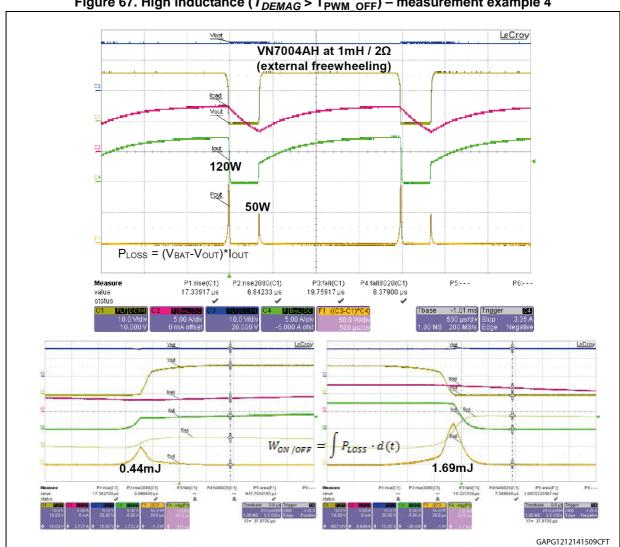
Measured losses (1 mH at 2  $\Omega$ ):  $W_{ON} \sim$  0.44 mJ,  $W_{OFF} \sim$  1.69 mJ
