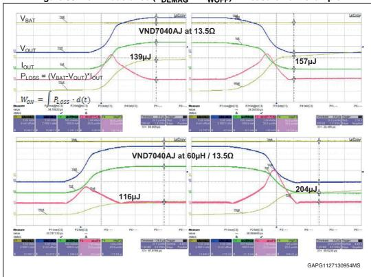
Figure 59. Low inductance (T<sub>DEMAG</sub> << t<sub>WOFF</sub>) – measurement example
