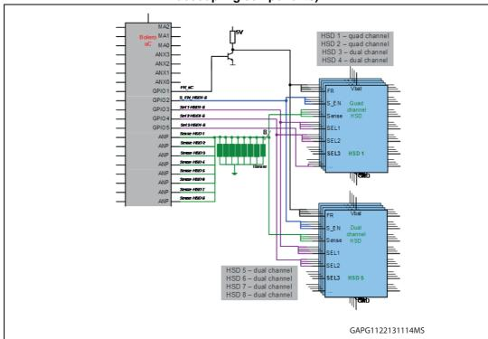
Figure 32. Common FaultRST pin handling example – basic schematic (without decoupling components)
