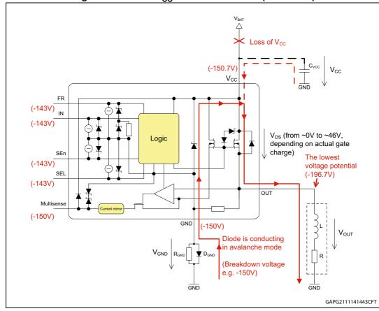
Figure 83. Loss of V<sub>CC</sub> with inductive load (monolithic)
