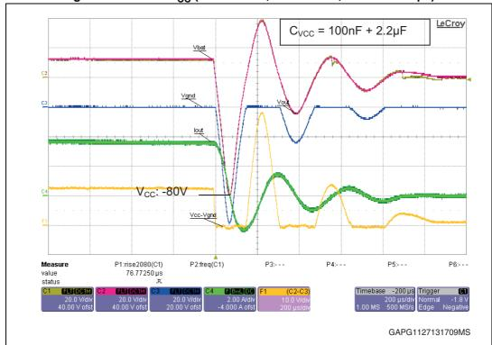
Figure 86. Loss of V<sub>CC</sub> (VND7020AJ, 1 mH/ 3.5  $\Omega$ , 100 nF + 2.2  $\mu$ F)
