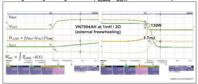
Measured losses (1 mH at 2  $\Omega$ ):  $W_{ON} \sim$  0.04 mJ,  $W_{OFF} \sim$  1.75 mJ
