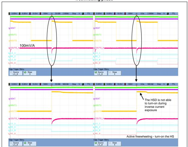
Another example with one VND7012AY and two VNB35NV04-E is shown in *Figure 165*. As seen from the measurement, the HSD is not able to turn-on during the freewheeling phase when the demagnetization current flows to the battery line via the body diode (same behavior as in case on monolithic device in previous example). Therefore, no active freewheeling is possible.
