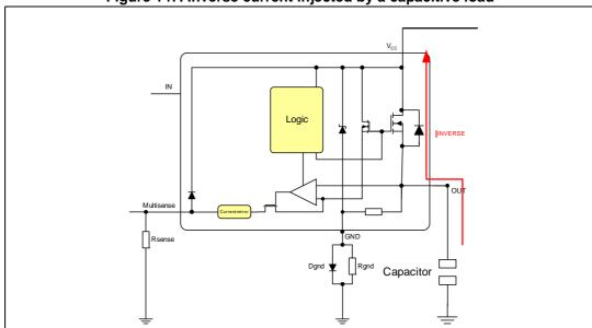
Figure 147. Inverse current injected by a capacitive load
