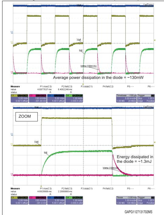
Figure 79. PWM 50% at 100 Hz, 2 mH / 5.5 Ω (VND7040AJ)
