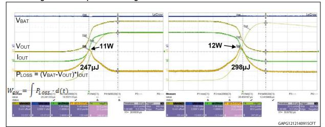
Figure 53. Example of switching losses on VNQ7040AY with 5.2  $\Omega$  resistive load
