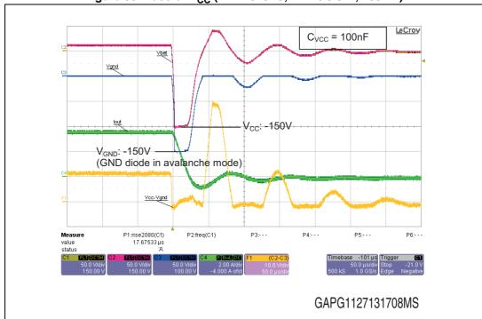
Figure 85. Loss of  $V_{CC}$  (VND7020AJ, 1 mH/ 3.5  $\Omega$ , 100 nF)
