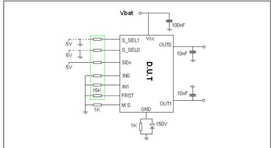
Figure 153. ESD test application scheme for HSD placed on a powered module
