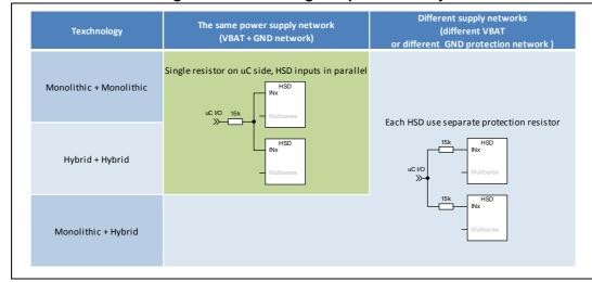
Figure 128. Paralleling of inputs summary
