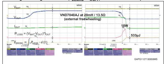
Figure 64. High inductance (T<sub>DEMAG</sub> > t<sub>WOFF</sub>): measurement example 1
