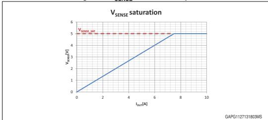
Figure 90. V<sub>SENSE</sub> saturation example
