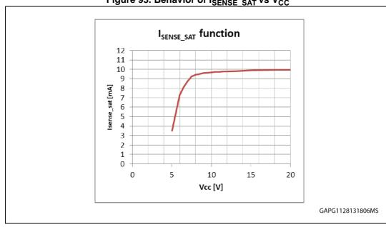
Figure 93. Behavior of I<sub>SENSE SAT</sub> vs V<sub>CC</sub>
