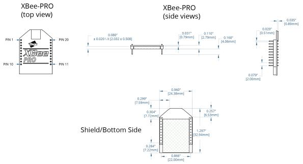
The following figure shows mechanical drawings for the RPSMA variant of the XBee-PRO RF Module.
