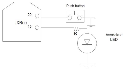
A pushbutton and an LED can be connected to module pins 20 and 15, respectively, to support the commissioning pushbutton and associated LED functionalities.
