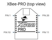
The following table contains pin assignments for the XBee/XBee-PRO RF Modules. (Low-asserted signals have a horizontal line above signal name.)
