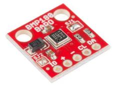
The BMP180 Breakout is a barometric pressure sensor with an  $I^2C$  ("Wire") interface.
