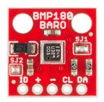
We'll connect four of the five pins on the board to your Arduino. The four pins you need are labeled +, -, CL, and DA.
