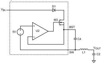
Figure 5—Internal Bootstrap Charging Circuit
