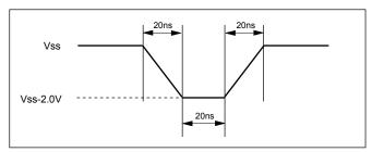
**Figure 3. Maximum Positive Overshoot Waveform**
