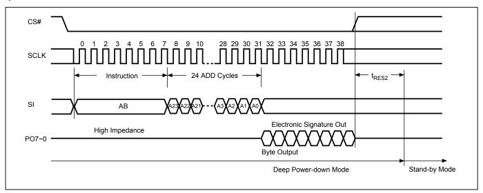
Note: Under parallel mode, the fastest access clock freg. will be changed to 6MHz(SCLK pin clock freg.)
