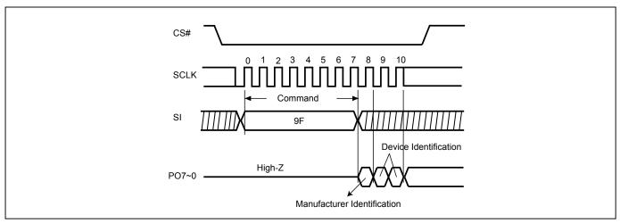
**Note:** There are 3 data bytes which would be output sequentially for Manufacturer and Device ID 1'st byte (Memory Type) and Device ID 2'nd byte (Memory Density).
