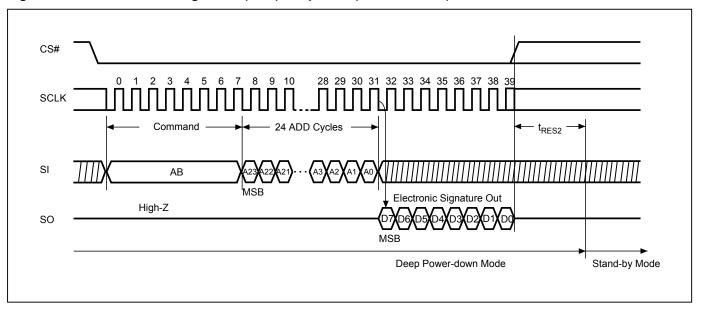
Figure 34. Release from Deep Power-down (RDP) Sequence (Command AB)
