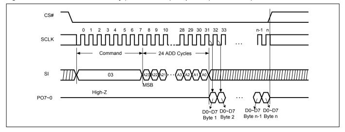
Figure 31-7. Parallel Mode Page Program (Parallel PP) Sequence (Command 02)
