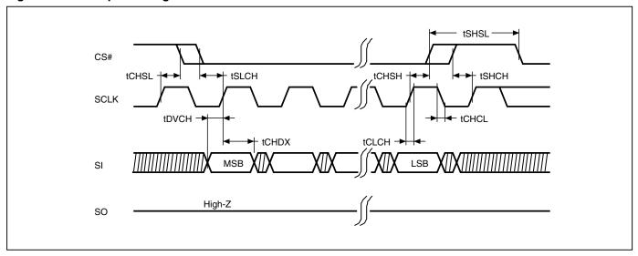
Figure 7. Output Timing
