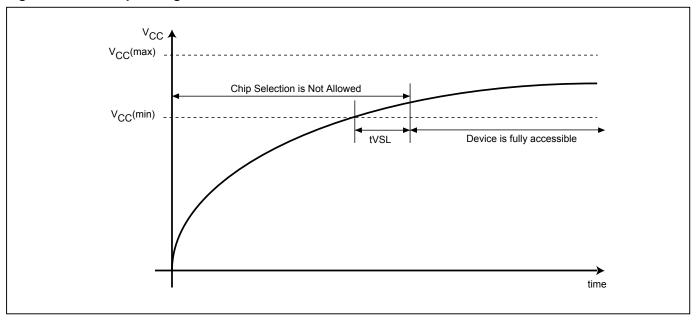
Note: VCC (max.) is 3.6V and VCC (min.) is 2.7V.
