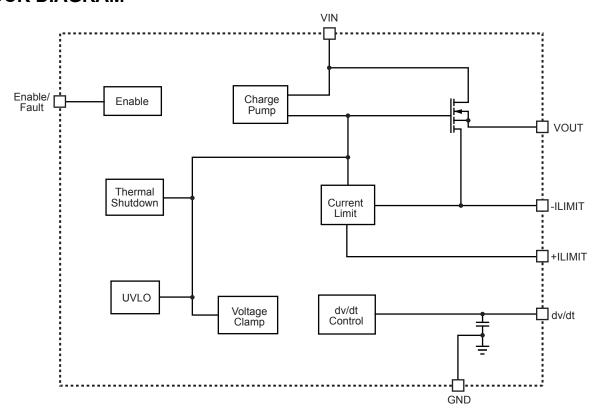
Figure 1—Function Block Diagram
