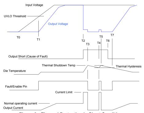
Figure 3—Thermal Protection in Short Condition
